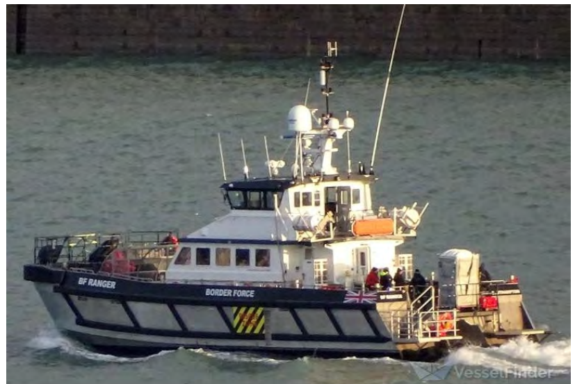
BF Ranger, one of 5 crew transfer vessels, designed to support the offshore wind turbine industry and adapted to 'rescue' large numbers of illegal migrants from the middle of the English Channel, from inflatable boats, before landing them at Dover. Modifications include the provision of a portable toilet on the aft deck.
